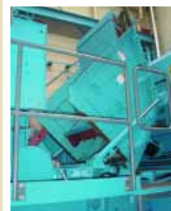
▲ CHAIN CURTAIN Full width single strand chain curtain.
