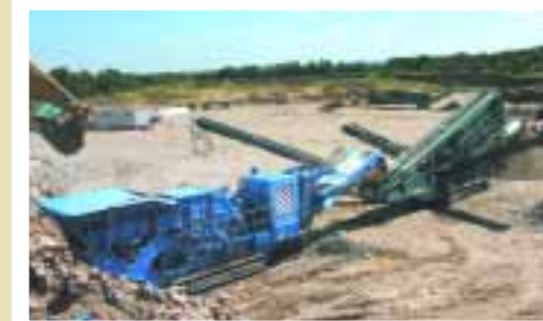
▲ 1412 Trakpactor feeding a Powerscreen 2400 Chieftain producing four grades of material.
