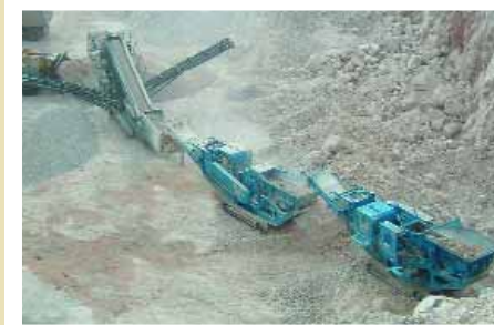
▲ 1165 Premiertrak feeding into a 428 Trakpactor feeding into a Powerscreen Chieftain in a quarrying application.
