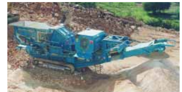
▲ A 428 Trakpactor working on a construction project producing crushed limestone at 300tph.
