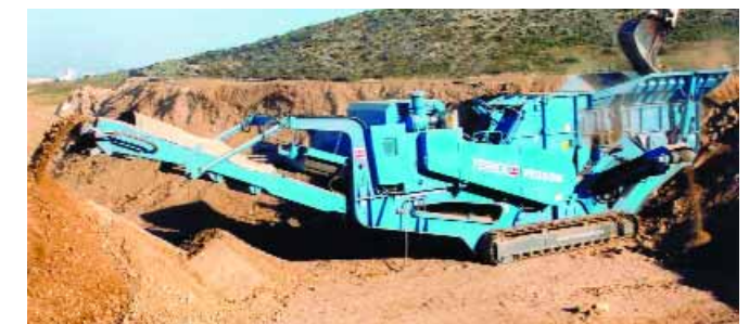
▶ A 1412 Trakpactor producing sub-base material at 550tph.
