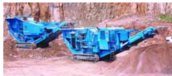
▲ 1165 Premiertrak feeding into a 428 Trakpactor in a limestone quarry.
